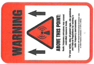
② WARNING - RF SIGN 12" x 18" DIGITAL PRINT MOUNTED TO 0.40 THICK ALUMINUM (OPERATIONS PROVIDED)
